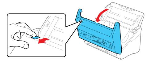
4. Use a genuine Epson cleaning kit or a soft, moist cloth to wipe off any dust or dirt on the glass scanning surfaces and the rollers inside the scanner cover. If the glass surface is stained with grease or some other hard-to-remove material, use a genuine Epson cleaning kit. Use a small amount of cleaner on the cleaning cloth to remove the stains. Be sure to wipe off all remaining liquid.
