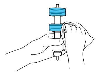
**Caution:** Use only a genuine Epson cleaning kit or soft, moist cloth to clean the roller; using a dry cloth may damage the surface of the roller. Do not spray cleaners directly inside the product; always spray cleaners on a cleaning cloth to slightly dampen the cloth. Wipe off any excess cleaner with a dry, lint-free cloth.
