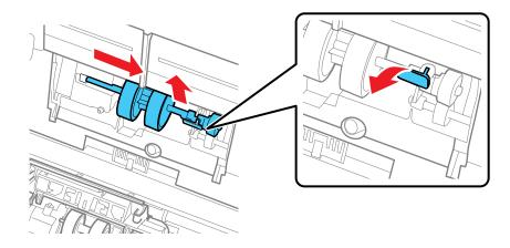
15. Wipe off any dust or dirt on the pickup roller using a genuine Epson cleaning kit or a soft, moist cloth.
