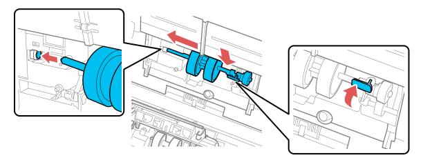
8. Align the bottom edge of the pickup roller cover into the notches as shown and press it down until it clicks into place.
