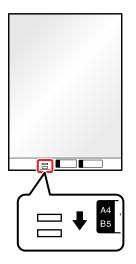
• For a Letter- or A4-size or larger original, fold it as shown and place it in the center of an optional carrier sheet. Make sure the illustration on the front edge of the carrier sheet is facing up.
