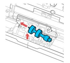
11. To install a new separation roller, insert the end of the roller into the hole on the right side and lower the other end of the roller into place.
