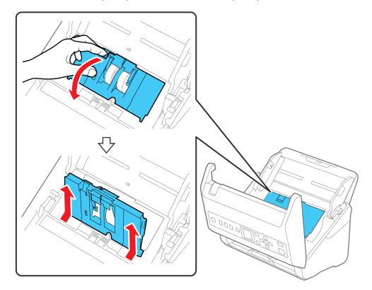
13. Press down on the pickup roller cover latch and pull up the cover to remove it.
