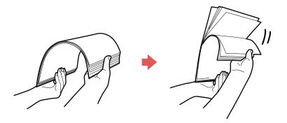
5. Stack the originals with the printed side facing down and slide the stack so the leading edge is at an angle as shown.
