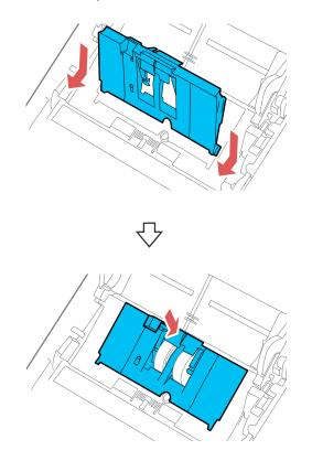
**Note:** If you are not able to close the cover, the pickup roller is not installed correctly. Remove the roller unit and reinstall it, then try to close the cover again.
