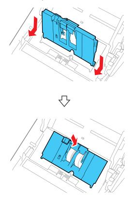
**Note:** If you are not able to close the cover, the roller is not installed correctly. Remove the roller unit and reinstall it, then try to close the cover again.
