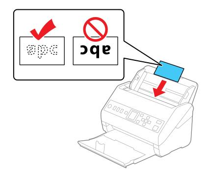
• If you are loading hole-punched originals, load them with the holes facing down or to the side as shown. The holes must be within 1.2 inches (30 mm) of the edge of the originals.
