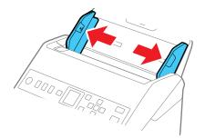
3. Load plastic or laminated cards (printed side down and long edge first) into the input tray horizontally, and slide them in until they meet resistance.
