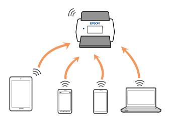
The scanner can be connected by Wi-Fi or Ethernet, and Wi-Fi Direct (Simple AP) connection simultaneously. However, if you start a network connection in Wi-Fi Direct (Simple AP) connection when the scanner is connected by Wi-Fi, the Wi-Fi is temporarily disconnected.
