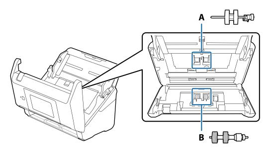
A: pickup roller, B: separation roller
