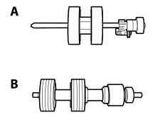
A: pickup roller, B: separation roller
