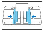
3. Place the card face down with the top edge at the bottom of the tray.
