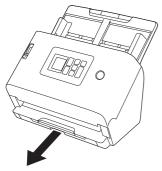
The document eject tray can be adjusted to 3 lengths. Pull out the document eject tray according to the length of the document. Also, erect the document eject stopper on the front edge if necessary.
