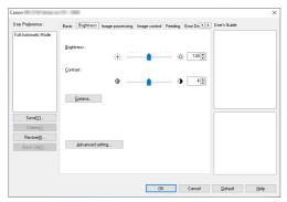
Adjust the brightness and contrast of scanned images. In addition, you can also click [Gamma] and set the gamma correction value for scanned images.
