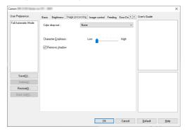
Set the processing method for scanned images.
