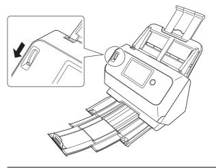
4 Adjust the document guides to fit the width of the document to be scanned.
