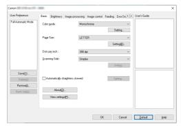
Configure basic scanning conditions such as the mode, page size, resolution, and scanning side.
