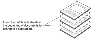
In an application, specify a patchcode as a type of batch separation.
