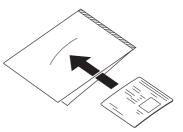
Load the document with the sealed end of the carrier sheet as the leading edge.
