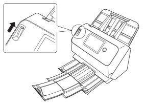
2 Adjust the document guides to fit the width of the card to be scanned.
