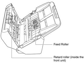
When closing the front unit, make sure that it is completely closed by gently pressing the left and right until you hear a click.
