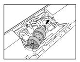
Push the left side of the retard roller to secure it to the scanner.
