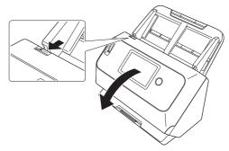
Use compressed air to remove dust and paper particles from the inside of the scanner.
