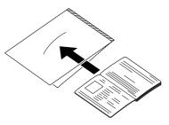
Load the document with the sealed end of the carrier sheet as the leading edge and the page you want to scan facing down.
