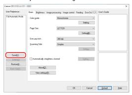
The saved setting is registered to the list. You can delete a setting from the list with the [Delete] button, and save or load a configuration file with the [Back Up] or [Restore] button.
