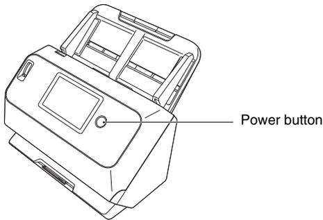
The power button lights blue when the power turns ON.
